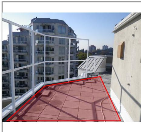
*Example: concrete pavers as a dead load.*
